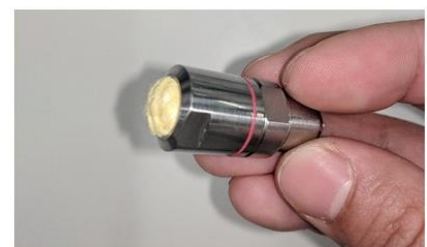
Proposed methodology for constant repeatability between the contact surface and the wiping cloth
