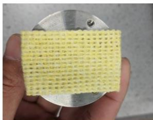
Flat Specimen self levelling sample holder, with the wiping cloth screwed onto it.
